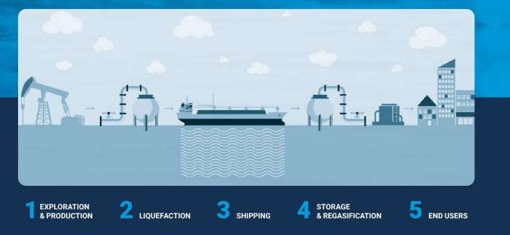
Access to energy is vital for economic and social development, and natural gas is one of the mainstays in the global energy mix. Liquefied natural gas (LNG) is natural gas that has been cooled down to liquid form for ease and safety of non-pressurized storage or transport. It is odorless, colorless, non-toxic and non-corrosive. The liquefaction process involves removal of certain components, such as dust, acid gases, helium water and heavy hydrocarbons.
